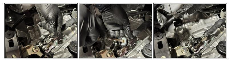
• Like the last bushing, remove the retaining clip. Slide the cable off the gear selector and use a tool to pry the bushing out.
