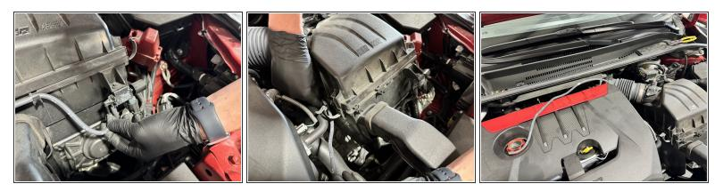
• On the front of the airbox, disconnect the vacuum line. You may need to use a pair of pliers.
