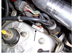
3. Unsnap the cruise control (if equipped) and throttle cables from their bracket near the driver side shock tower. Push the cruise control (lower) cable below the bracket and snap the throttle (upper) cable into the lower position on the bracket as shown in the figure below.
