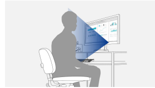
Sensor identifies a person at the workstation
