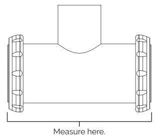
ThreadFit™ 30i: Installed on a 68mm bottom bracket shell the ThreadFit™ 30i is compatible with road BB30 type cranksets. Installed on a 73mm bottom bracket shell it is comaptible with mountain BB30 type cranksets.
