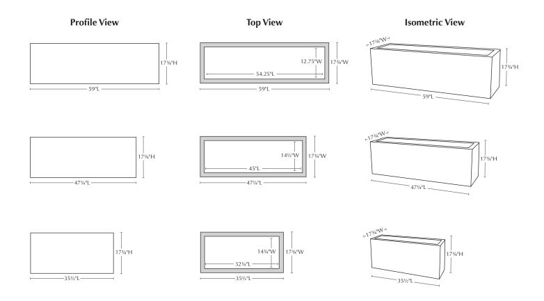
Materials: unsaturated polyester resin, sand, stone powder, talc powder, and fiberglass
