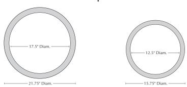
Materials: unsaturated polyester resin, sand, stone powder, talc powder, and fiberglass
