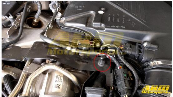
STEP 9: Disconnect the topside O2 sensors using an O2 sensor socket and remove them and their copper
