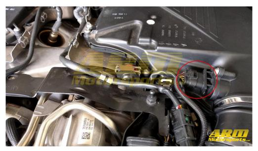
STEP 4: Disconnect the lower air tube on the air filter box. This is can be done by using a flat head screwdriver to pull the plastic away from the clip shown in the image.
