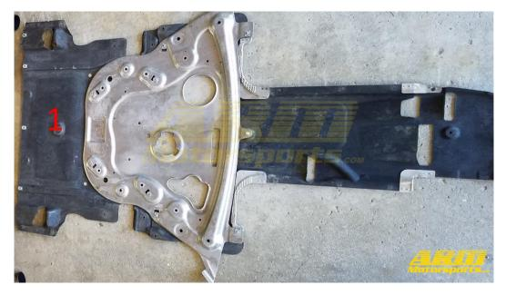
STEP 17: With this section of the undertray removed the metal splash guard is exposed. This is held on with 13mm bolts. When all the bolts are removed slide it towards the rear of the vehicle for it to drop
