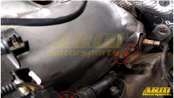
STEP 11: There are an additional 3 on the back side. In total there are 9 bolts which need to be removed. Once they are removed the heat shield can be lifted out.
