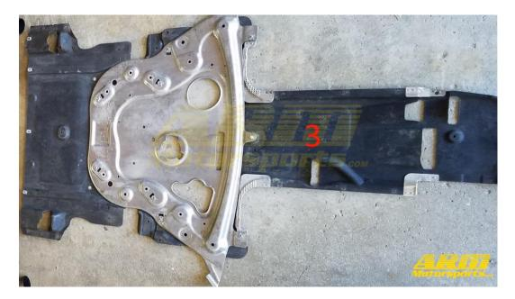
STEP 19: Now we have access to the clamp connecting the downpipe to the midpipe. Use a deep 15mm socket to loosen this on each side.
