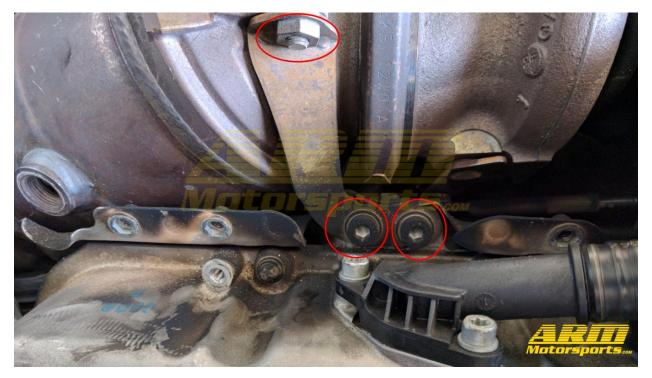
STEP 13: There are another two 6mm hex bolts on each side holding the downpipe to the back of the engine which need to be removed.
