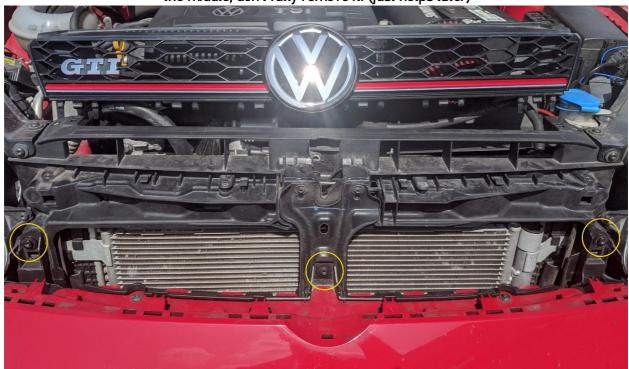
The intercooler brackets will be mounted in between these two plastic bolts holes.
