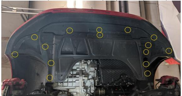
Remove the skid plate by pressing the front tabs to release it. Then the fender liners should just fall out with it.
