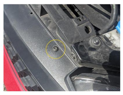
2. While your still here, remove the two T25 torx screws that hold the bumper to the upper cross support.
