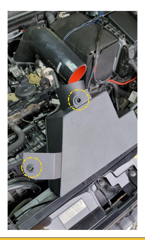
At this point you get to make a decision for what clamp you want to use, the filter will use its supplied worm clamp. For the silicone to airbox clamp, we include both a worm
