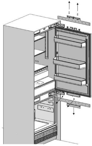
• Remove the panel adjustment mechanisms from the lower part of the freezer door.
