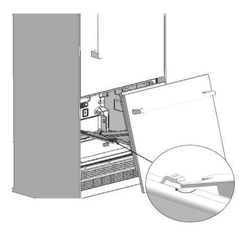
Fix the freezer door panel assembly onto the rails with the two • screws removed earlier.
