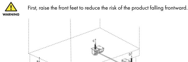
A/D –Turn the key clockwise to lift the front B/C –Turn the key clockwise to lift the rear
