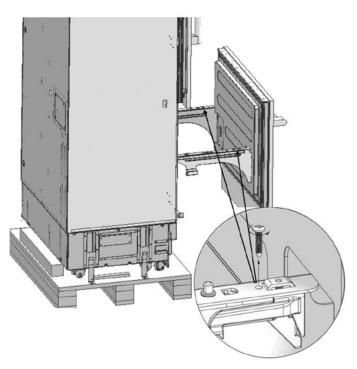
While supporting the freezer door, pull it forward while freeing it from the rear rail lock tabs to remove it.
