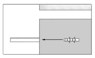
Fit the brackets (Item No. 7) into their places, using four screws for each. • You must use both brackets to ensure safety of the product.
