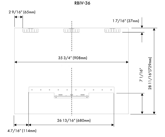
Handle connection holes must be adjusted according to the handle orientation you plan to use in your kitchen design.
