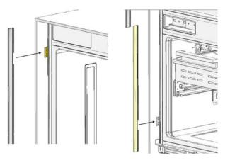
• Attach the upper closing part (Item No. 4) onto the connection bracket.
