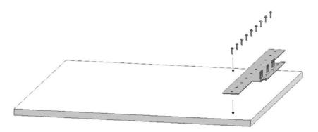
• Attach three sheet metal brackets (Item No. 25) using six screws (Item No. 15) for each.
