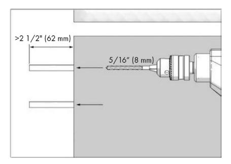
Use the hammer to fit the anchors (Item No. 8).
