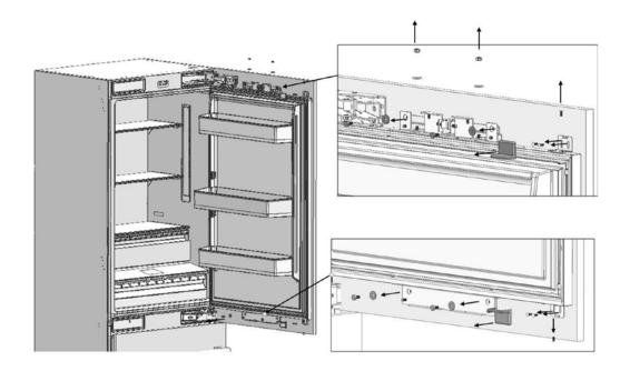
• Remove the screw of upper and lower mechanisms.
