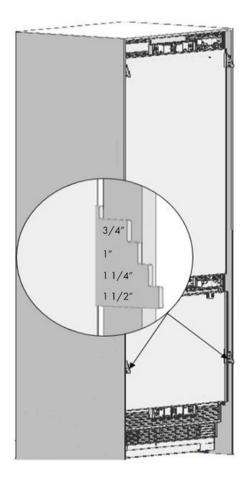
• The position of the position alignment gauge (Item No. 10) must be adjusted according to the thickness of the door. It can adjust the level for four different door thickness levels.
