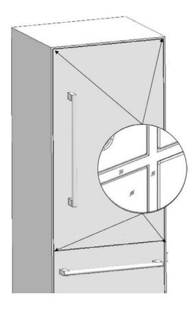
• For products without clad doors, the product is placed using the position alignment gauge (Item No. 10) as shown in the figure above.
