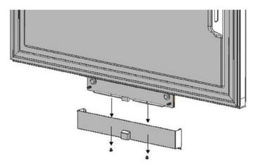
• Remove lower and upper bracket screws.
