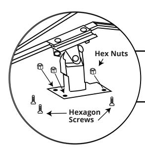
After installing the transition fitting, attach the motor component to the bottom plate using hex nuts and hexagon screws. Tighten the screws to complete installation.
