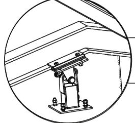
According to the diagram, install the transition fitting on the steel I-beam, and then lock the fastening screws to complete the installation.
