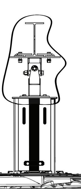
The next step in the installation process includes using the provided wire rope, locks, and tiger claws to stabilize and secure the fan to the building structure. See the diagram below for proper placement using the supplied fan parts identified below.
