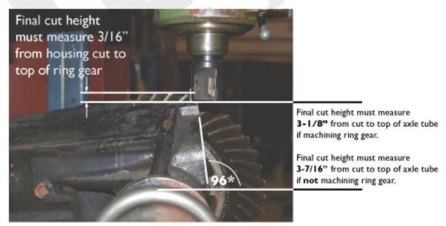
Step 6: Bolt the differential cover to the housing and cut the differential cover down at 90 degrees to the housing so the height of the diff cover matches up evenly with the height of the housing.
