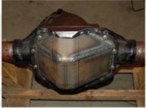
Step 12: Check for any clearance issues and modify housing/differential cover/shave plates if required.
