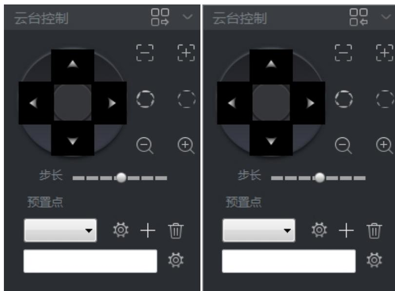
PTZ control interface unfolds (left) and expands (right)
