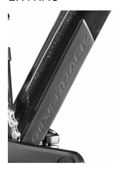
Downtube protector included on frame to reduce rock strike damage to paint and frame in critical area and also helps to reduce noise of impacts.
