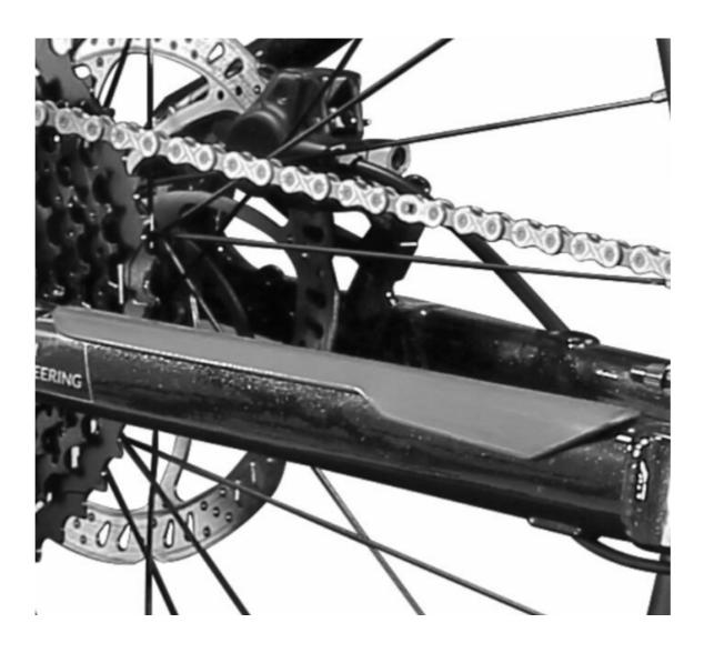
Silverback chainstay protector included to help dampen chain slap on chainstay and protect tubing.
