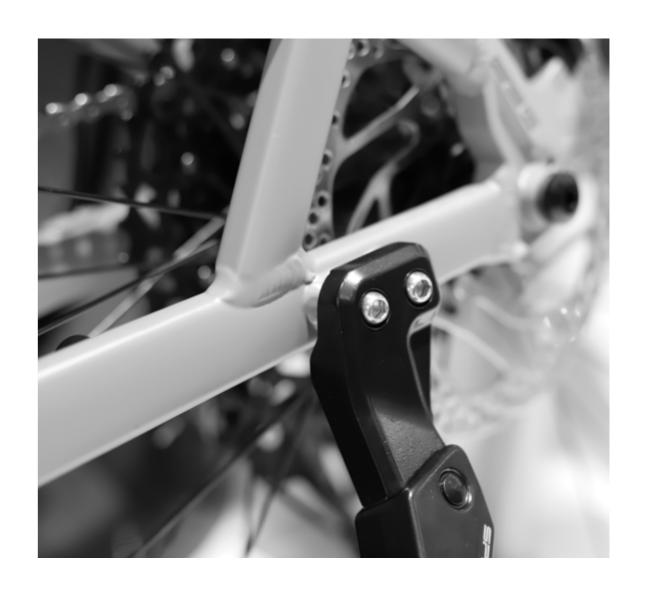
Integrated 18mm kickstand mount for best secure attachment.
