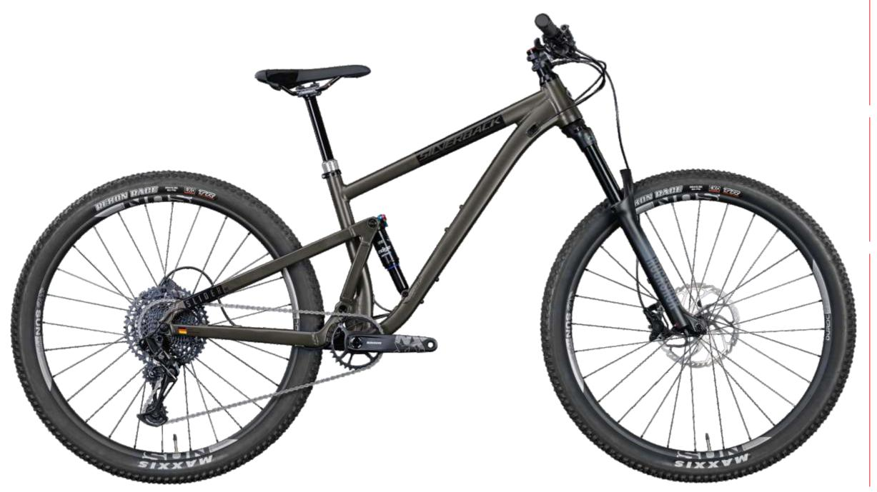
Frame New Slider Hydro-formed 6061-T6 Alloy Frame. 150mm travel,
