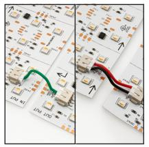
Use the 1.6" green (data) connectors to link two LED sheets for synchronized color changing.
