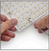
Use the 6" cables to link the LED sheet to the power supply or contoller.
