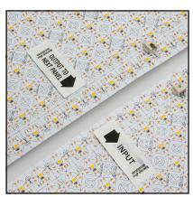
Ensure you check the polarity of the connectors; otherwise, the light will not turn on. Pay attention to the input and output decals on each sheet. These decals must be removed after installation.
