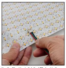
Use the 6" cables to link the LED sheet to the power supply or contoller.
