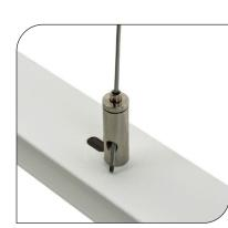
• Fasten the gripper into the track channel using the provided screw, and feed the cable through the gripper hole. Adjust the height by pushing the cable holder down.
