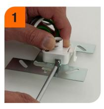
• To separate the track connector from the mounting plate, simply loosen the two screws.
