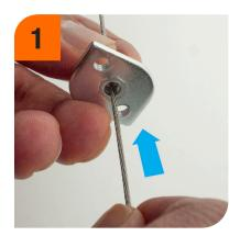
Insert the suspension cable into the designated cable holder.
