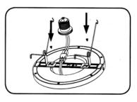
Remove trim and existing lamp from recessed fixtrue.
