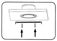
Fixing bracket on terminal box.
