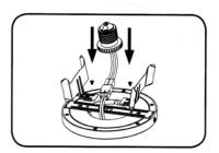
Remove trim and existing lamp from recessed fixtrue.
