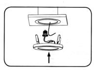
Screw E26 scoket adapter into scoket in the housing.
