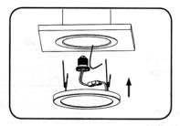
Screw E26 scoket adapter into scoket in the housing.
