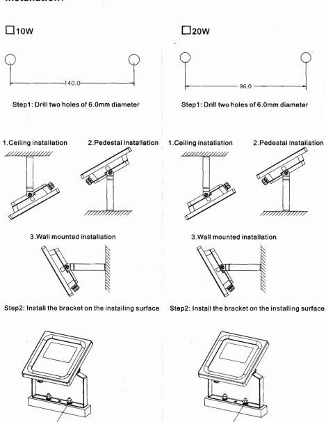
Step3: Fix the bracket and light together with bolts and nuts Step3: Fix the bracket and light together with bolts and nuts
