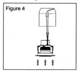
Step 8: Make sure the trim of LED Lamp is fitted into recessed housing in ceiling firmly.
