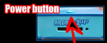
On your Mega Man Console, press the power button so that it is in the on position.
