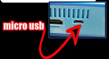
Once you have both the USB plugged into your computer, and the Micro USB plugged into the Mea Man Console, go back to your Flash Tool. At the bottom of your Flash Tool, the status should have changed from "No Devices Found" to "Found One MASKROM Device."
