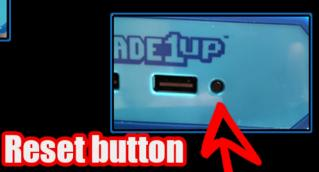
Locate the reset button on the front of the console. Once located you want to press and hold the reset button down.
