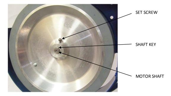
Once the set screw is loosened, slide the wheel off the end of the motor shaft. If it does not come off easily, you may need to use a wheel-puller to get it off. Some WD-40 may also help. DO NOT hit the wheel with anything to get it off. This would damage the motor.
