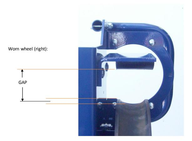
If, for example, if the wheel has 3/8" of wear, divide the total wear (3/8") by 2, that gives you 3/16". So, you would need to reduce the GAP by a total of 3/16". There are a couple of different ways to accomplish this.
