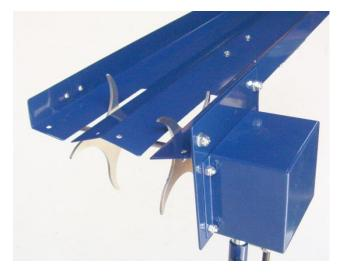
Attach the Motor assembly to the Feeder Tray (as shown left) using the 10-24 x 5/8" Phillips screws, washers, and lock nuts.
