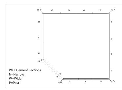
**STEP 2** - Locate the wall elements (sections). There are two sizes. The narrow element sections (N) are approximately 17" wide and will be used to construct the short walls that connect to the door. The wide element sections (W) are approximately 19" wide and will construct the two long walls.
