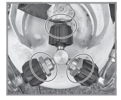
If parts of the fitting begin to produce bubbles, spray liquid, or if you smell liquid propane gas, immediately close the valve on the tank. Wait 5 minutes for any gas to dissipate. After waiting for 5 minutes, the leak(s) must be stopped by tightening the loose joints, if possible, or by replacing the faulty part(s) with the part(s) recommended by the appliance manufacturer.
