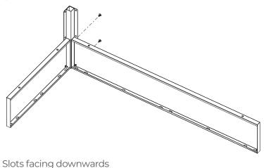
1c. Affix 1 x corner post (part 5) to the opposing end of the long bottom panel using  $2 \times M5 \times 12$  screws (part 7)
