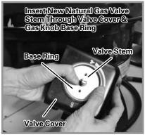
Align the openings of the valve, valve cover and control knob seat and insert the two screws.
