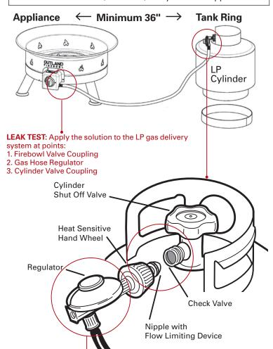
**LEAK TEST:** Apply the solution to the LP gas delivery system at points. Valve coupling regulator & Cylinder Coupling.
