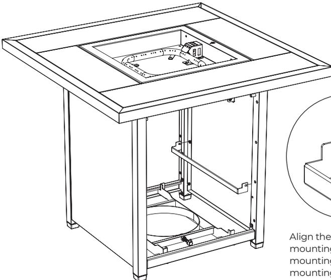
Align the open slots of the mounting brackets with the mounting screws. Push the mounting bracket forward until it can't move further in. Tighten both mounting screws.
