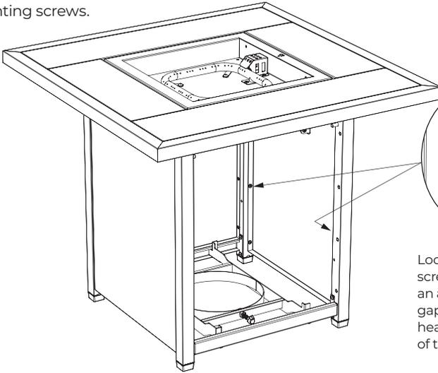
Loosen the screws with a screwdriver until there is an approximately 3 mm gap between the screw head and the side flange of the panel.
