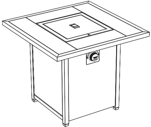
**Note:** It may be necessary to adjust the position of glass rocks to have the lid sit flush on the fire table.
