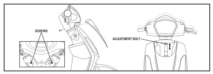
Figure 14. Tiller Height Adjustment
