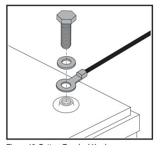
Figure 12. Battery Terminal Hardware
