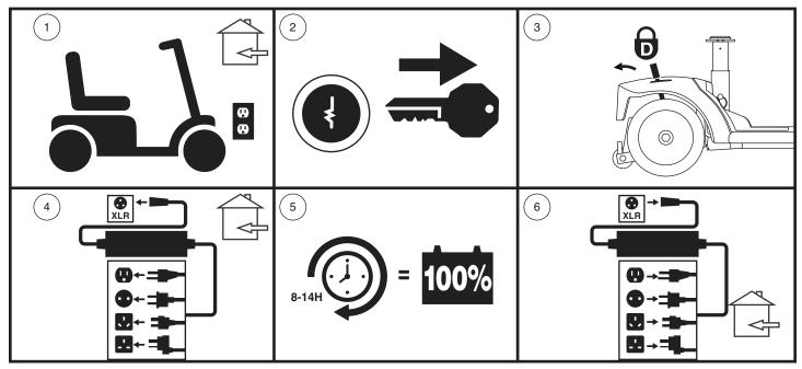
Figure 9. Battery Charging Procedures Diagram
