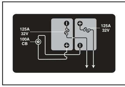
Figure 11. Battery Configuration
