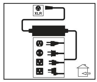
Figure 3. Off-board Battery Charger
