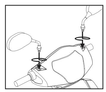
Figure 15. Mirror Position Installation/Adjustment
