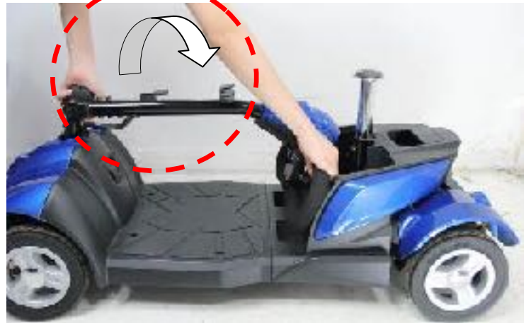
8. Loosen the tiller adjustment knob and fold down the tiller and retighten knob.
