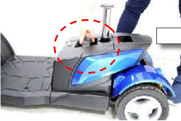
7. Pick up the battery pack and remove it from the scooter.
