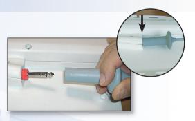
2. Hang the hand control on the backrest. Push the cable at the end of the hand controller onto the jack in the back of the backrest. Make sure that the cable is properly seated on the jack. The red ring at the jack is now unseen.
