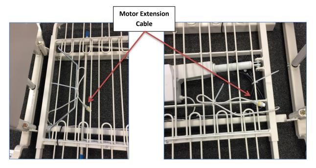
9. Plug the motor extension cable into the high low actuators. Then install the "C-Clips" that are in the bag with the user manual, these should lock in place (Step 4). Followed by, fastening the remaining cord to a washer with a tie strap provided.
