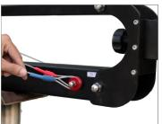
**NOTE:** You can adjust the cable with help of wire tensioner.
