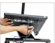
• Lastly, insert the bolts into the Base Platform to secure the LCD monitor with it.
