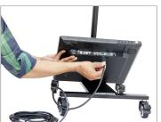
• Now, connect the power adapter cable to the respective port.
