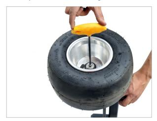
• Insert the push bar handle into the Rear-Wheel Steering and lock it with the provided pin.
