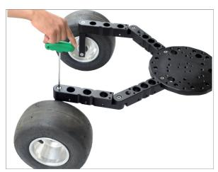
**NOTE:** Pull the pin of the Wheel Steering and you can adjust the direction of the tyres. (front tyres remain fixed)
