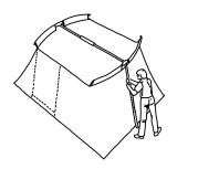
2. Insert Ridge Poles and Spring Bars. Use 2 ridge poles, 1 steel sleeve, and 4 spring bars.
