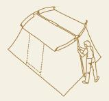
2. Insert Ridge Poles and Tension Rods. Use ridge poles (three piece), 1 aluminum sleeve, and 4 tension bars.
