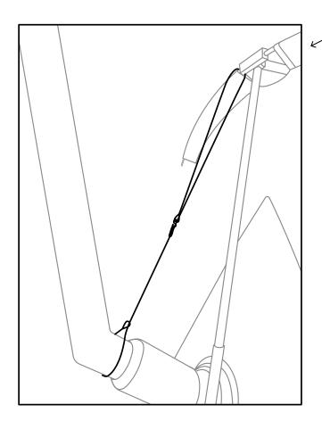
7) Attach Springbar® Chimney Support Cable.
