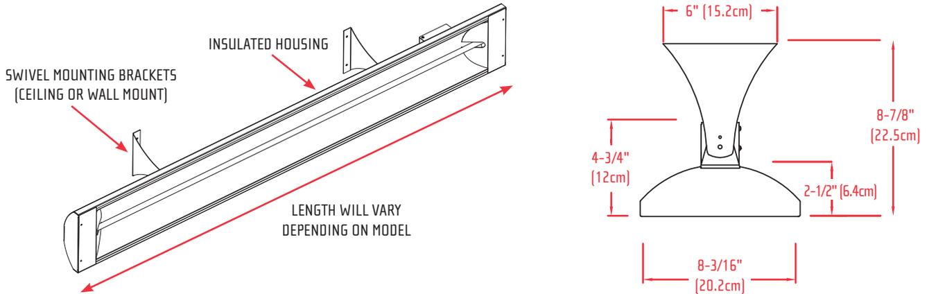
Heater must be installed with the quartz tube horizontally level. For maximum tube life, use a carpenter's level tool to find the optimum level position for the heater's body. It's important to always maintain the minimum clearances from the heater body to any combustible materials.
