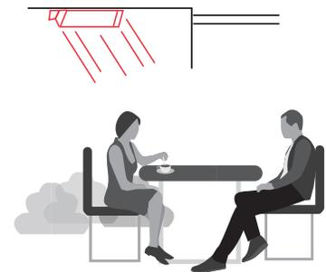
When outdoors, hang heater under protective roof or weather cover whenever possible. Even though heater is all-weather construction, it will last longer and look better if it is protected from rain and snow.
