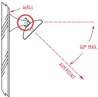
Detail of C-Series Multi-Position Mounting Bracket Tab
