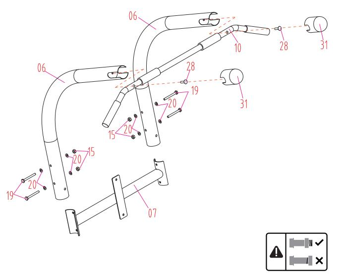
With the help of an assistant, slide the L Shaped Upper Frames (#06) into the Uprights (#05) as oriented in illustration indicated below. Insert two Bolts (#25) through two Curved Washers (#20) followed by the VKR Arm Rest Support
