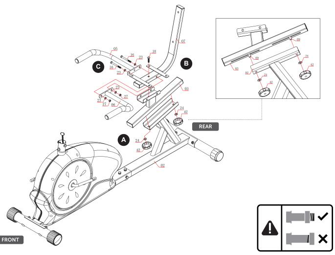
Remove the pre-assembled parts from the Main Frame (#01) and set them aside: three Bolts (#17), three Spring Washers (#25) and three Arc Washers (#26).
