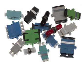
Fibre Couplers allow connections at each end and are typically used in patch panels, wall boxes and surface boxes. Applications include enterprise, data centre, LAN, FTTx and Telecom. Available as LC, SC, ST and FC versions in multimode, singlemode and APC versions. LC and SC couplers are colour coded to define the fibre type with singlemode in blue, multimode OM3 or OM4 Aqua and OM4 in Heather Violet. APC connectors are green.
