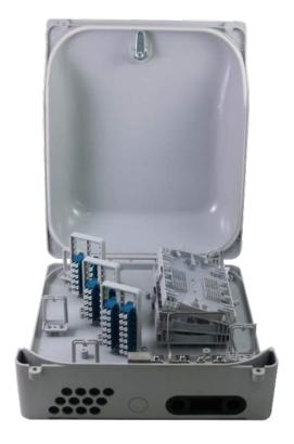
xSiCute IP65 rated moulded plastic external connection box for up to 108 fibres. Suitable for use as a breakout box or a splice enclosure. The patching area accepts up to 54 x LC duplex couplers or 54 x SC simplex couplers. Supplied with 3 x 24 position fibre splice trays and can accept an additional three trays if required. Trays are hinged to allow access to other trays and open beyond 90 degrees enabling unencumbered access to installed fibres. May be externally mounted on poles or walls.
