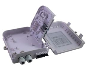
xSiCute IP65 rated moulded plastic external connection box is UV and weather resistant providing protection from dust and water ingress. Suitable for use as a breakout box or a splice enclosure. Supplied with 1 x 12 position built in splice tray and able to accept 12 x LC duplex or 12 x SC simplex couplers, (couplers not supplied with termination box). Suitable for external use and can be mounted on walls or poles.
