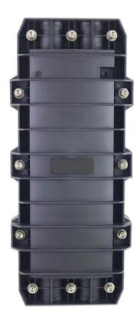
xSiCute IP68 rated moulded plastic external splice box suitable for protecting up to 96 fibre splice terminations. Supplied as standard with 1 x 24 fibre splice tray and will accept a further three trays as required. Trays are hinged to allow access to other trays and open beyond 90 degrees enabling unencumbered access to installed fibres. With a water-tight silicone seal, suitable for direct burial or wall mounting and resistant to UV and vibration.
