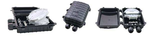
xSiCute compact IP68 rated moulded plastic external splice box suitable for protecting up to 48 fibre splice terminations. Supplied as standard with 2 x 12 position fibre splice tray and can accept an additional two trays if required. Trays are hinged to allow access to other trays and open beyond 90 degrees enabling unencumbered access to installed fibres. Resistant to vibration and UV with a water-tight seal suitable for direct burial. Can also be wall mounted.
