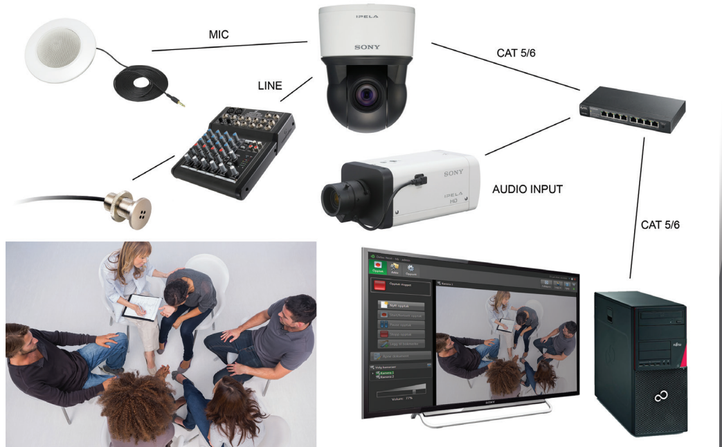
A Detec Record HD-system typically consists of 2-4 cameras (free number possible), where minimum one usually is a Pan-Tilt-Zoom camera. Microphones are connected via cameras. Cameras are connected via a network switch to an off-the-shelf PC for recordings.
