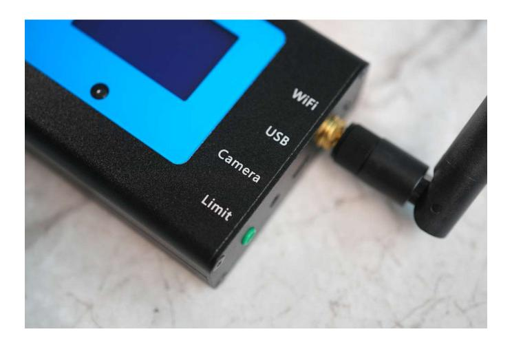
**Camera Port** -- this is where a camera shutter release cable is plugged in. It is a 2.5mm stereo socket which most of camera cable on the market supports. The tip for the camera port is for the camera trigger signal and the middle ring is for the focus signal.
